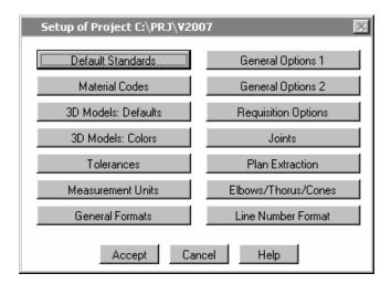
Selecting the Accept button all changes will be written in the \project\DBF\[project]SET.DBF table where the project setup is stored. Each button allows entering a specific set of parameters. Refer to the Help button in each dialog box to get a detailed information of each option.
