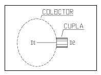
In all the cases, but the EOL (Elbolet) and LOL (Latrolet), the axis of the branch pipe makes an angle of 90 degree with the main pipe axis. In case of latrolets both axis make a 45 degree angle. In case of the Elbolet, this component only can be placed on an Elbow.
