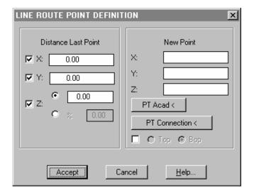
Each point can be specified by typing its absolute (relative to current UCS) X Y Z coordinates (in the **New Point** window) or in a relative way with respect to the last point (in the **Distance Last Point** window). The new point coordinates can also be graphically picked using an AutoCAD<sup>®</sup> point selection or a snap to a connection point of an existing component.
