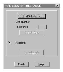
Selecting a pipe end, if it has already defined a length tolerance, this value will be displayed in the Tolerance field.
